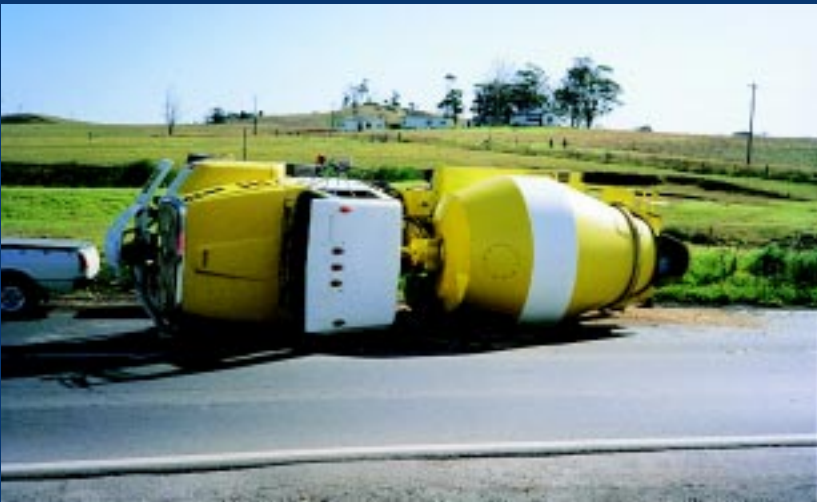
This vehicle lost a poorly restrained lightweight roll of plastic 'bubble wrap'. An oncoming concrete agitator rolled (see below), when swerving to avoid the obstacle on the road. (Photo courtesy Mick Simpson, Wales Truck Repairs).
