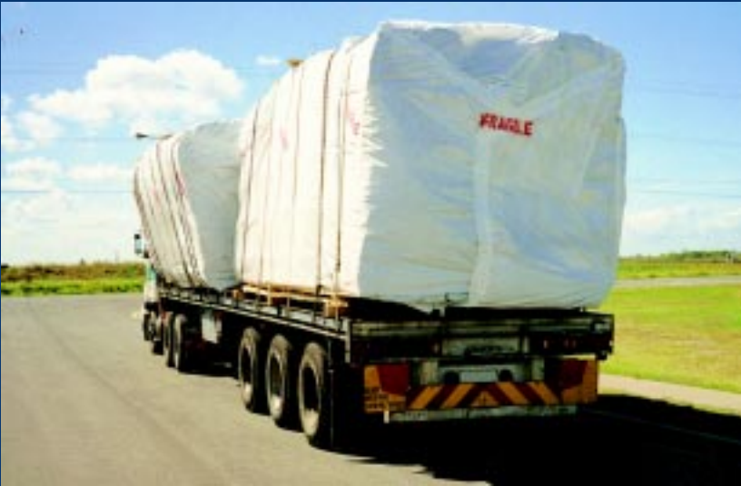
Lengths of timber slipped sideways after the load had settled on packing strips that separated the timber. (Photo courtesy Queensland Transport).
