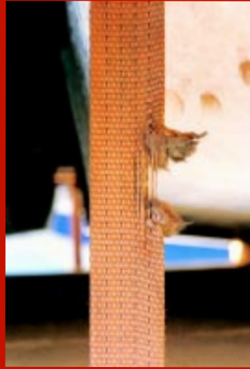
Typical damaged webbing straps (see Section H.2 for allowable wear).
