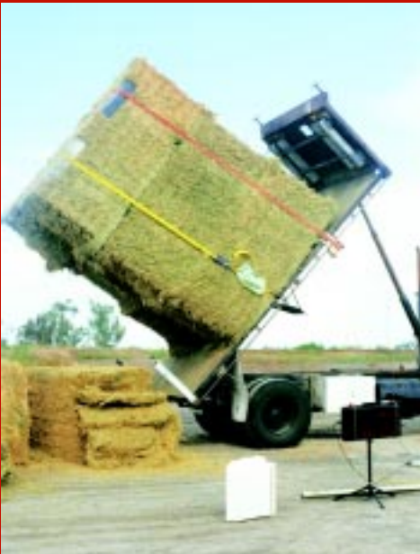
The solution was to use two straps and steel edge protectors. This allowed the bales to stay on the fully tilted truck. Without the edge protectors the webbing straps cut through the bales. With the protectors in place the straps could be fully tensioned.
