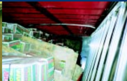
These photos show what happens to an unrestrained load in a curtain-sided trailer when it rolls over. (Photos courtesy Mick Simpson, Wales Truck Repairs).
