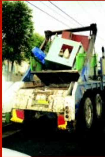
Loads in skips or tippers must be restrained if there is any possibility of the contents coming out.
