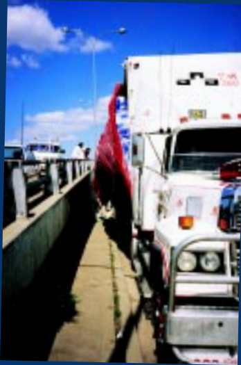
This photo shows a curtainside with a severe hernia. The load shifted on a corner. (Photo courtesy Mick Simpson, Wales Truck Repairs).
