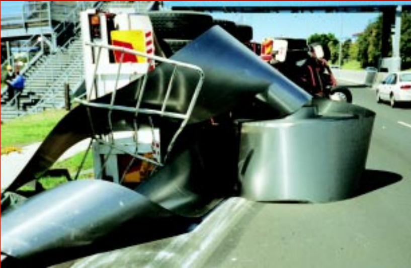
The steel straps on this 15 tonne steel coil broke allowing the centre of the coil to spear outwards, causing the trailer to roll over.
