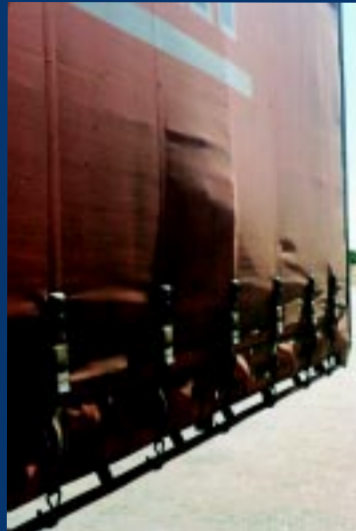
A bulge in a curtain can indicate that an unrestrained load is inside. The truck might also exceed the maximum width limit of 2.5 metres.
