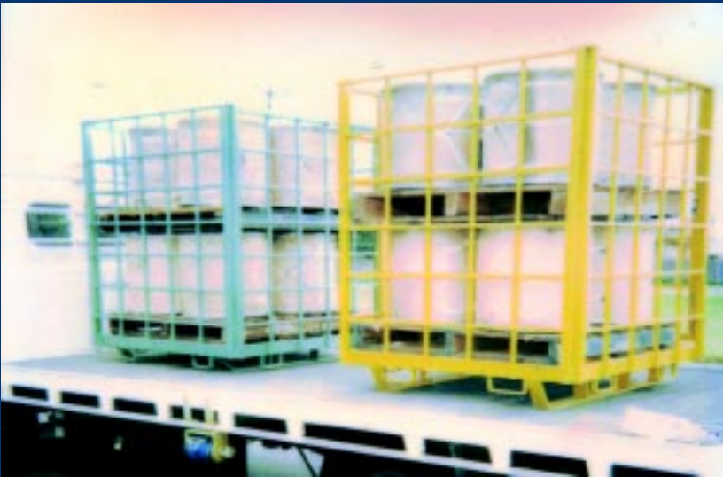
The product is well contained in the crates, but the crates aren't restrained on the truck. (Photo courtesy John Brentnall).
