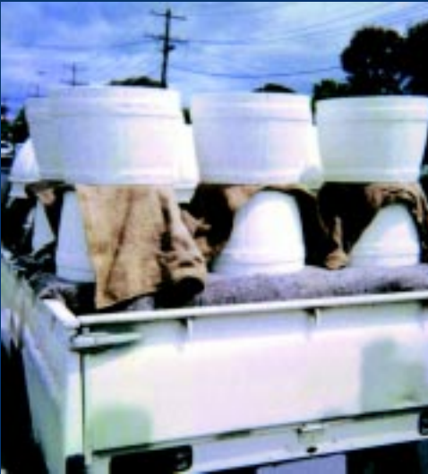
These concrete pots had no restraint at all! (Photo courtesy John Brentnall).
