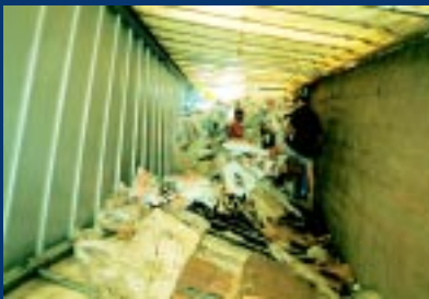
These photos show what happens to an unrestrained load in a curtain-sided trailer when it rolls over. (Photos courtesy Mick Simpson, Wales Truck Repairs).
