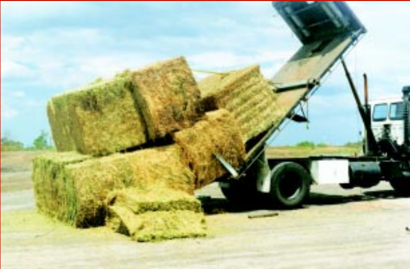
Load testing large hay bales (2.4 m x 1.2 m x 1.2 m). In this case only one webbing strap per row was used and the bales collapsed.
