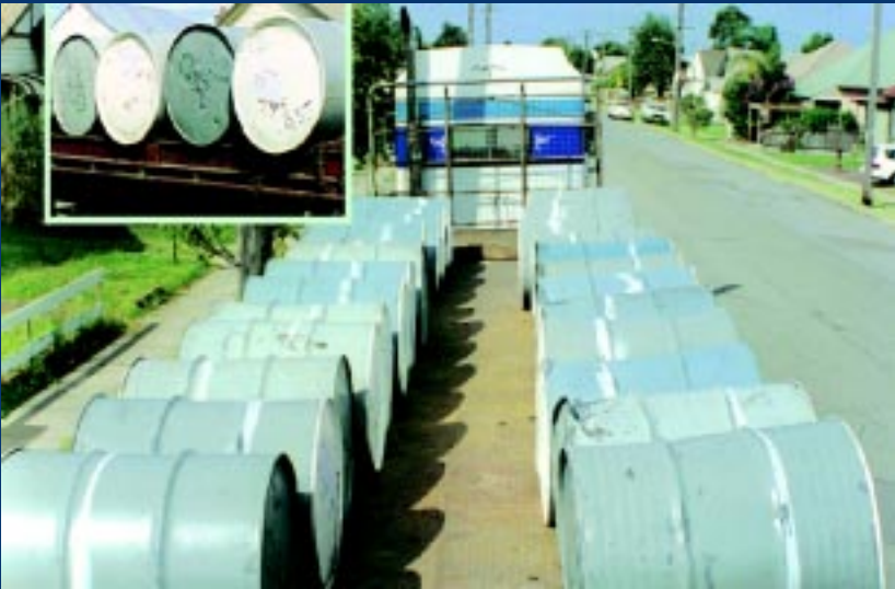
These 26 drums are filled with ball bearings and weigh almost one tonne each. None are restrained. Note that the drums overhang the coaming rails making it even easier for them to fall off in a corner (see photo insert).
