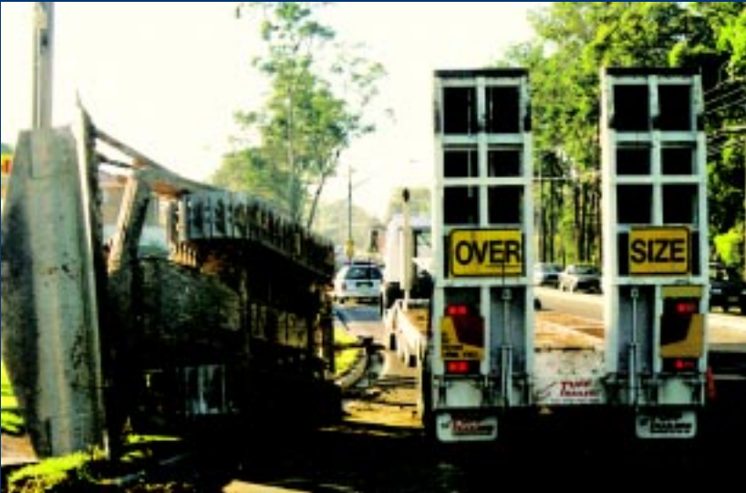
This bulldozer was not restrained and slid sideways off the low-loader. Steel on steel is low friction and therefore high risk.
