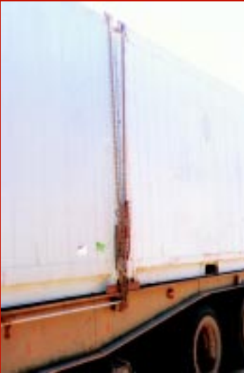
Chains can be used to secure freight containers although in this case where two chains are used, check the anchor point strength first.
