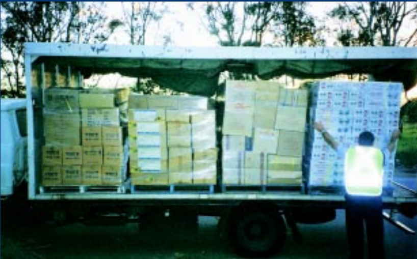
There were no lashings on this load and the plastic wrapping did not adequately hold the load together. (The enforcement officer is holding a leaning pallet of boxes on the truck while the driver is getting some restraint equipment from the toolbox).
