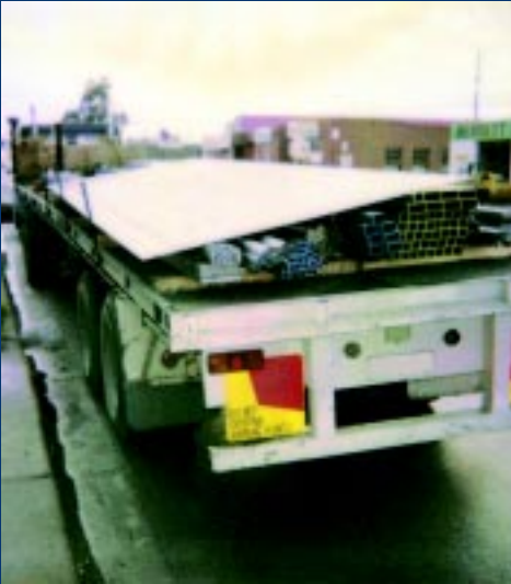
Airflow could lift and dislodge this large sheet. All of the load must be properly restrained. (Photo courtesy John Brentnall).
