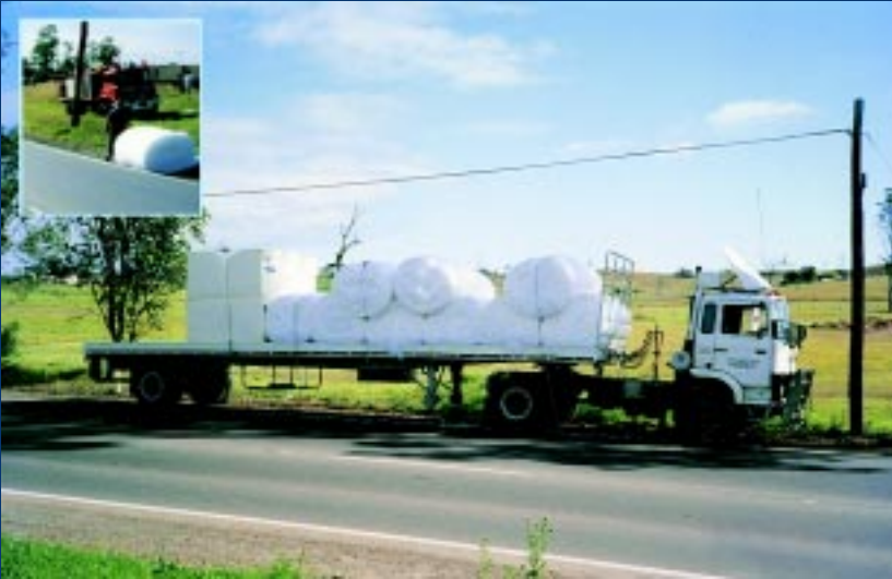
This vehicle lost a poorly restrained lightweight roll of plastic 'bubble wrap'. An oncoming concrete agitator rolled (see below), when swerving to avoid the obstacle on the road. (Photo courtesy Mick Simpson, Wales Truck Repairs).
