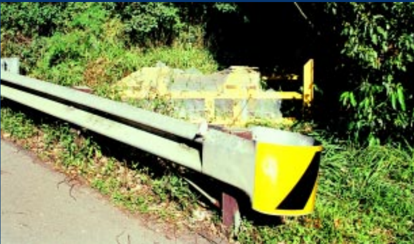
The driver was unaware that this new 1800 kg press, still in its plastic wrapping, had broken through a side curtain and fallen on the roadside. The press should have been tied in the trailer, with lashings arranged to stop it tipping over.
