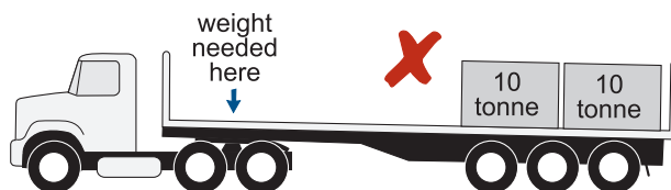
Fig. B.10 INSUFFICIENT WEIGHT ON DRIVE AXLES
