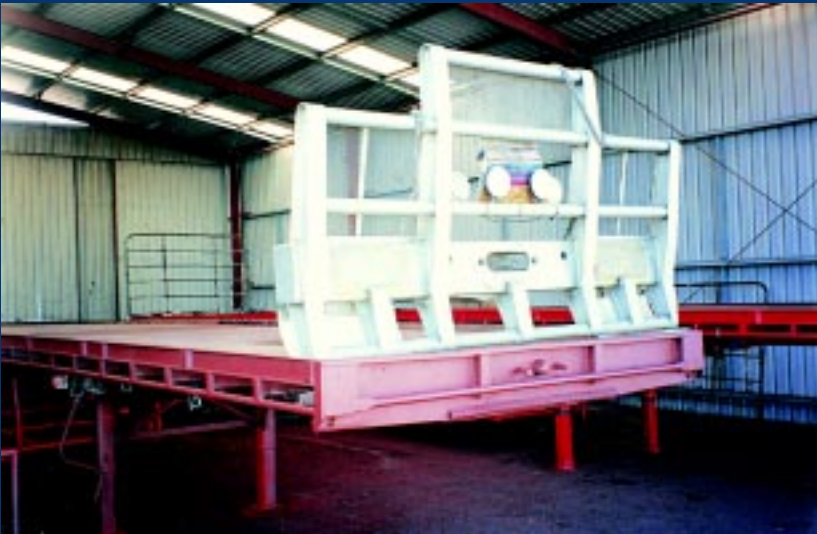
The strength of the bullbar could provide greater driver safety if placed at the front of the load (see page 73 and 74).
