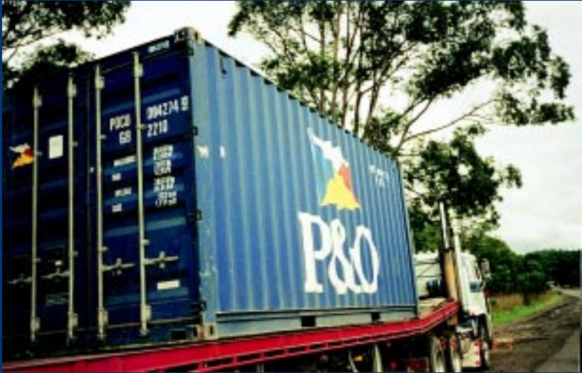
The shipping container bent this trailer. It is important to know the weight of the load and its centre of mass and then to position it correctly on the appropriate vehicle.
