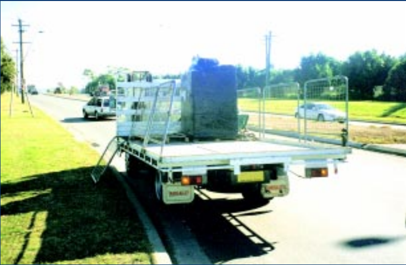
The lightweight load (below) bent the front left-hand gate (above) almost to the ground).
